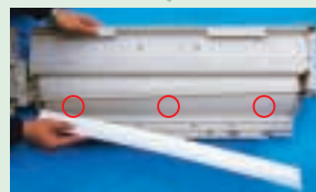
Polystyrene spot fused in the 2004-model (○: fused spots)
