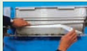
Foam polystyrene glued along the entire surface in the 2003-model
