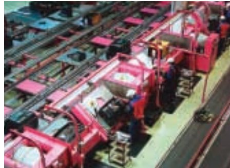
Dismantling used TVs at the Matsushita Eco Technology Center Photo 1
