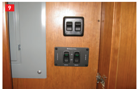
(7) Heat exchangers are strategically placed to provide the best distribution of warm air. (8) A common location for a heat exchanger is at the bottom of a cabinet drawer. (9) Switches for the system are installed in a central cabinet with other fifth-wheel controls.
