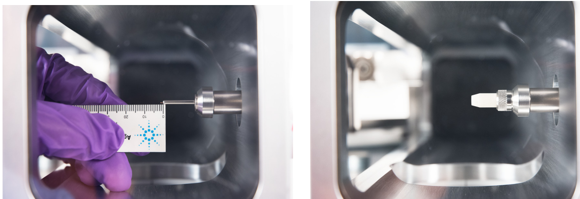
Figure 5. Installing a capillary column in the GC/MS interface for an EI EXT, SS, or Inert source.
