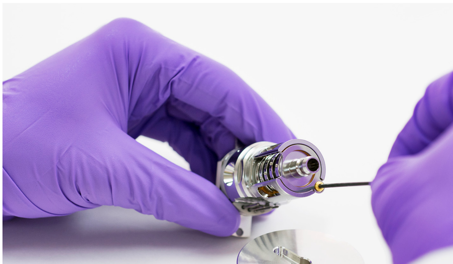
Figure 40. Secure the lens screw and lock ring insulator
