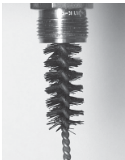
Figure 5-46. Cleaning the valve with the valve brush.
