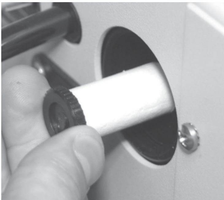
Figure 5-30. Removing the filter mount.
