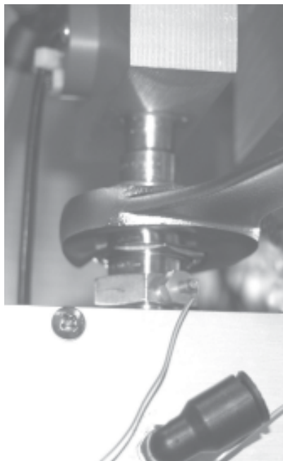
Figure 5-45. Removing a valve Swagelok fitting.
