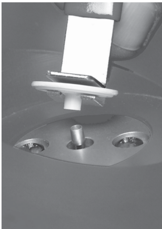
Figure 5-8. Placing the filter on the tapered element.
