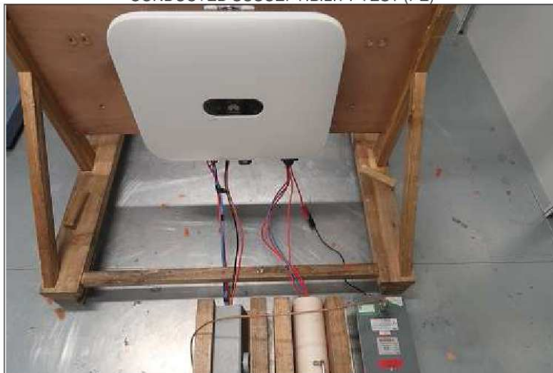
CONDUCTED SUSCEPTIBILITY TEST (PE)
