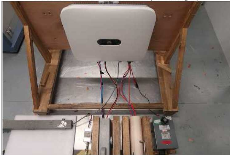
CONDUCTED SUSCEPTIBILITY TEST (Shielded Signal)
