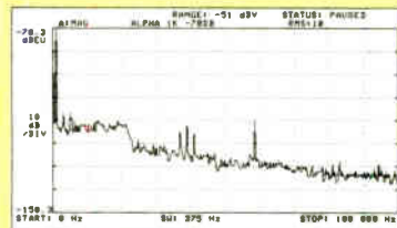
Fig 2. Arcam Alpha Plus: spurs up to 100kHz associated with 1kHz tone at -70\text{dB}
