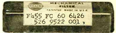
Fig. 7 This is the type of filter used to remove the unwanted sideband from the output signal.
