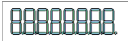
Figure A.79 Connected Parts Display Example (7-segment LED)
