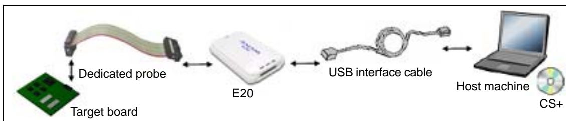
Figure 2.3 Connection Example [E20]
