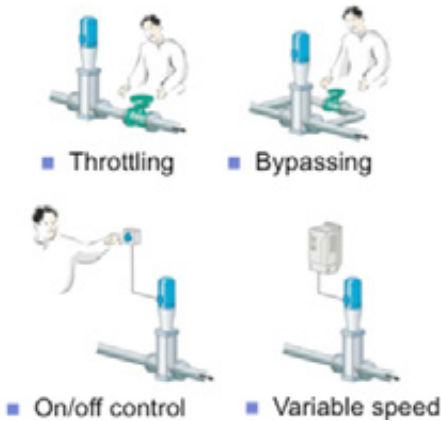
Figure 2.7 - Common flow control methods, (ABB Oy) Drives, 2006)
