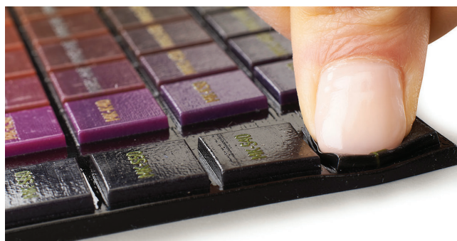
Figure 8. Various colors and Shore A values are displayed on this palette.
