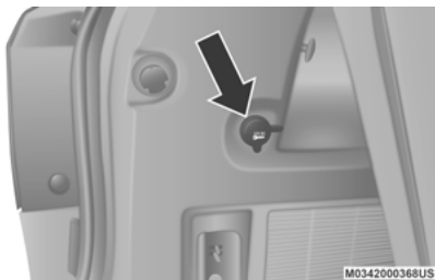
Rear Cargo Area Power Outlet
