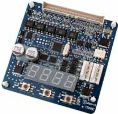
Figure 41. VelociTach motor control board
