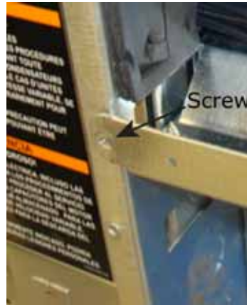
Figure 105. Fan board attachment screw
