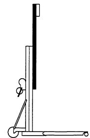
**CAUTION** Crushing hazard. Do not stand directly under columns.
