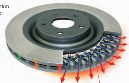
Improved cooling for increased disc rotor efficiency
