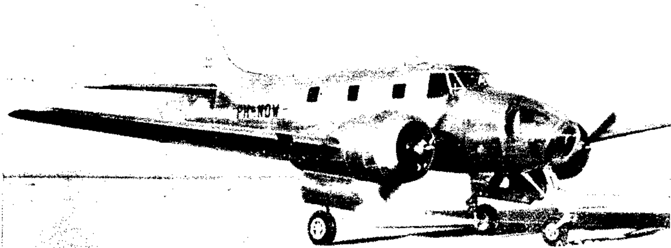
The Dutch Fokker S. 13, an advance trainer weighing more than 12,000 pounds loaded, is powered by 600 h. p. P & W Wasp engine.
