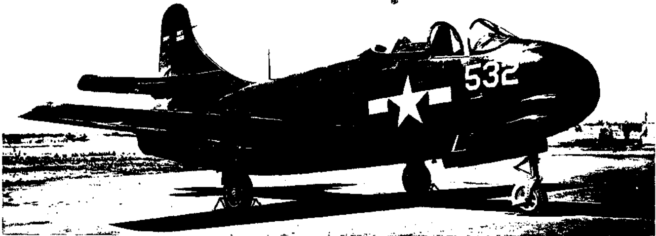
Designed by Chance Vought, the F6U PIRATE is a carrier-based jet fighter that has seen very little operational duty.
