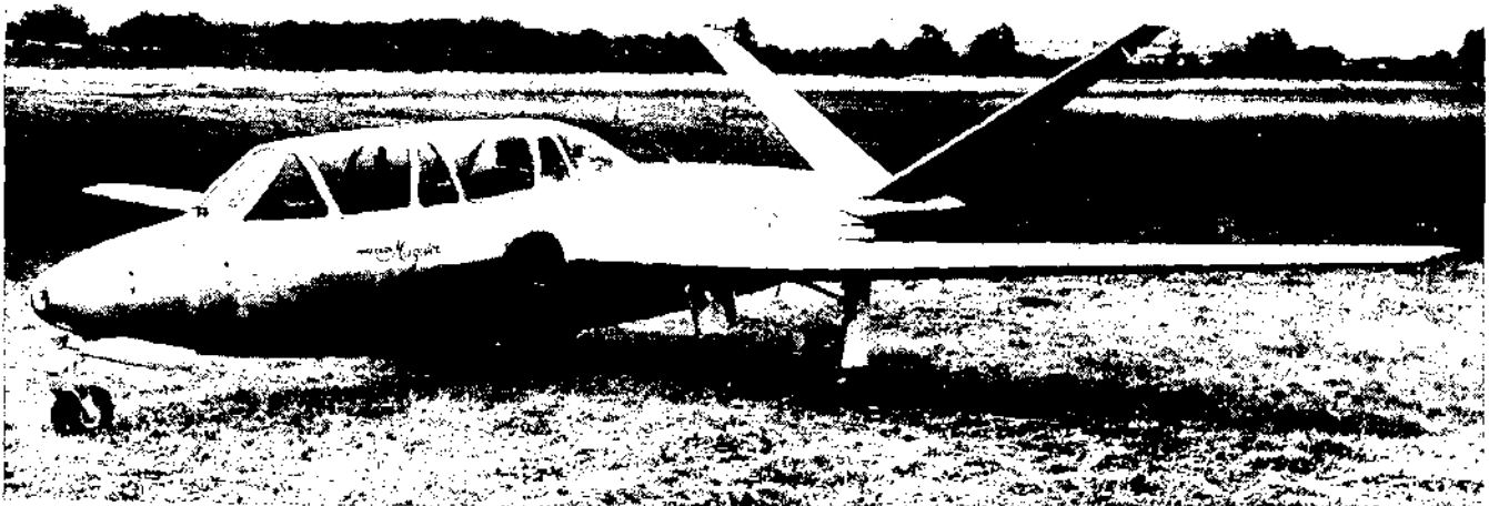
The French Fouga C.M. 170-R MAGISTOR is a two place, tandem type jet aircraft designed as a jet trainer for student pilots.
