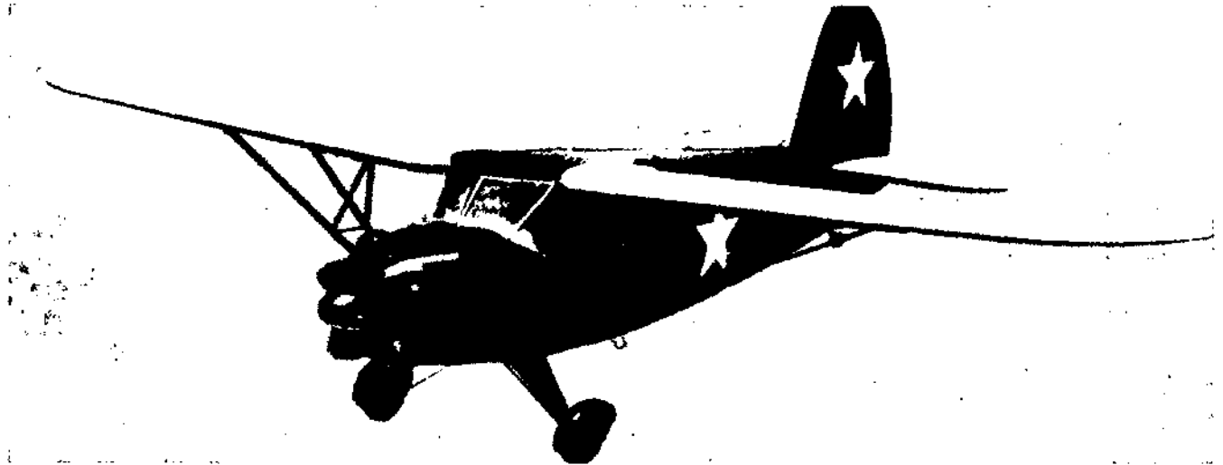
The Soviet "CROW" (Yak-14) is a strut-braced high-wing four-place monoplane with a fixed landing gear.
