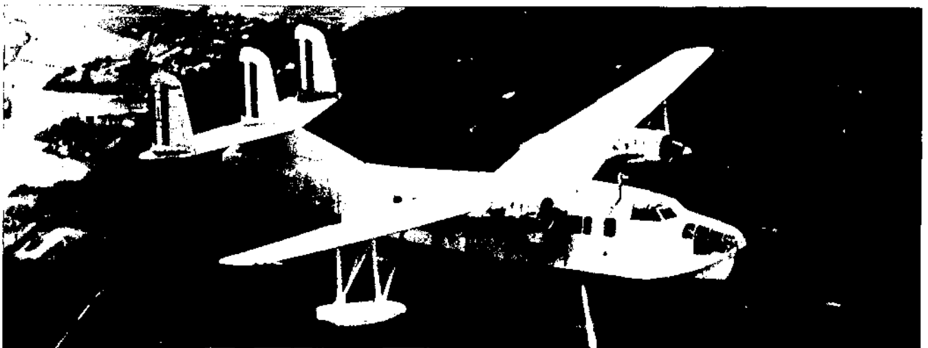
The Nord 1400 reconnaissance and rescue amphibian has been tested with different make engines and is in production for the French Navy.
