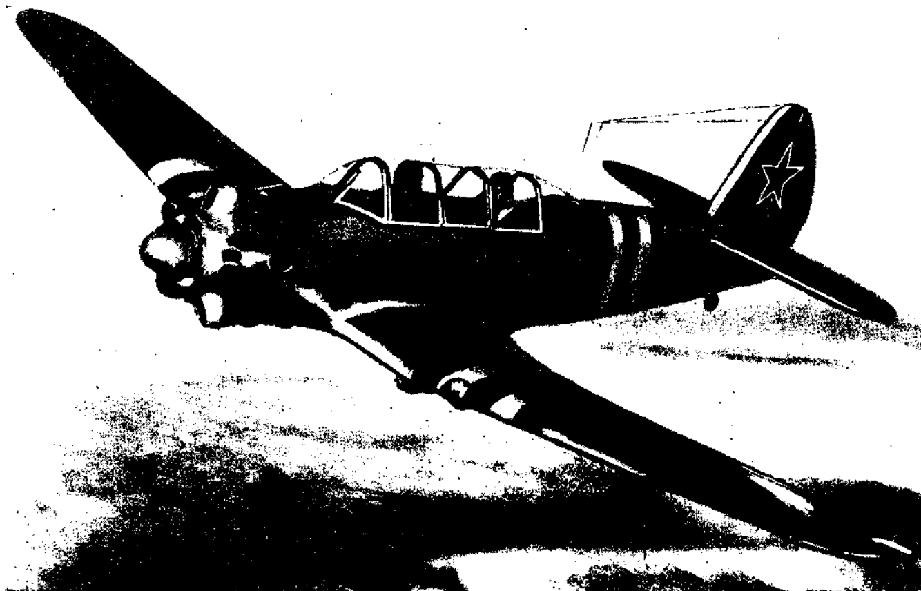
The Yak-18 is a single engine low-wing trainer featuring a radial engine with cylinder fairings, a tapering wing, and a fixed landing gear.
