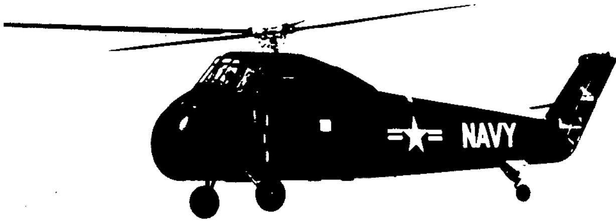
Sikorsky's XHSS-1, powered by a 1,425 h. p. R1820 engine, is a four-bladed, anti-torque rotor, anti-submarine helicopter.
