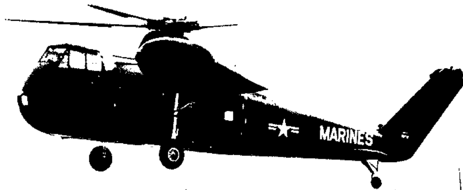
Sikorsky's XHR2S twin-engine helicopter has retractable landing gear and was designed for Marine transport duties.
