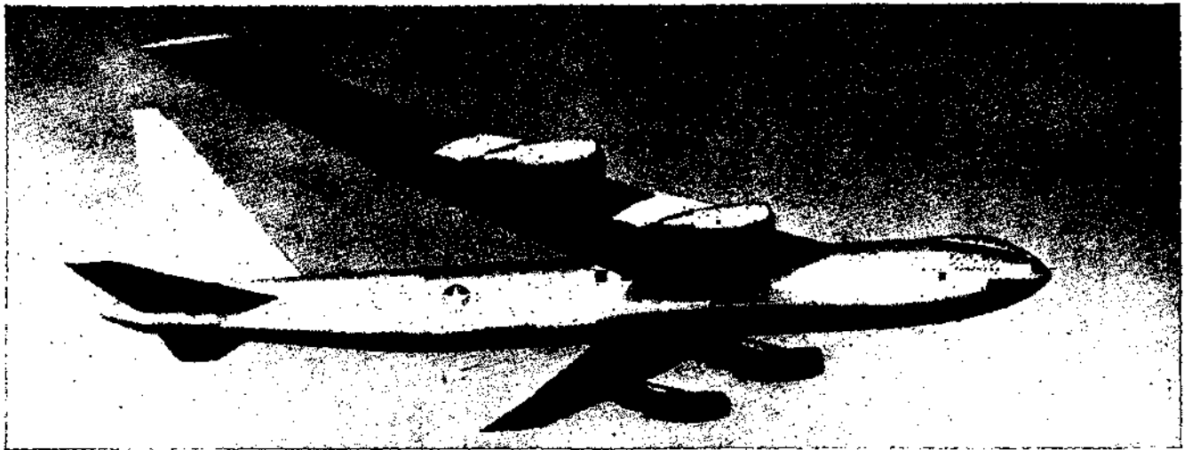
Boeing's YB-52 STRATOFORTRESS, a long range heavy bomber, features eight J-57 turbojet engines, and a decelerating parachute.
