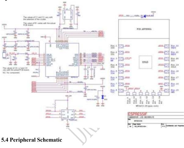
This is the typical application circuit of the module connected with peripheral components (for example, power supply, antenna, reset button, JTAG interface, and UART interface).
