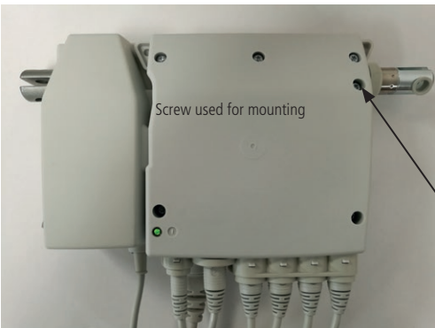
CB9 mounted on actuator, LA31.
