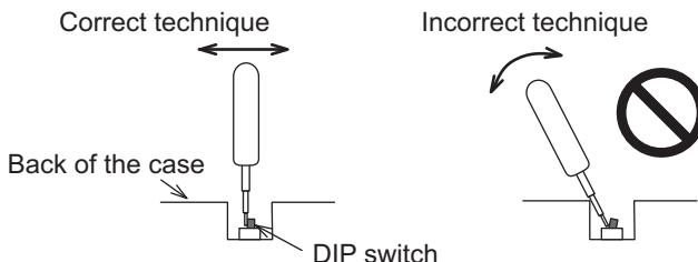
The DIP switch may break if it is levered with a tool against the case as shown in the figure.
