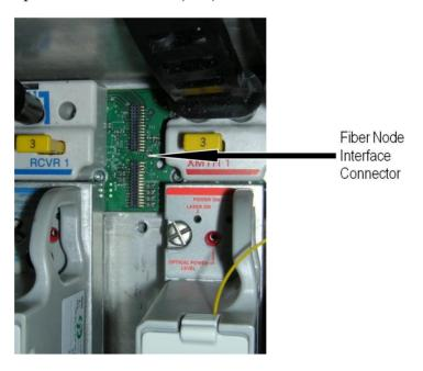
6 Push the transponder down firmly onto the OIB until the transponder seats into position. Use the screws provided with the transponder to secure the transponder to the board. The screw locations are shown in the following illustration. Tighten screws to 25-30 in-lbs (2.8-3.4 Nm).
