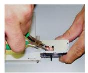
4 Position the transponder so that the interface connector shown below aligns with the node interface connector. This connector is located on the optical interface board (OIB) in the lid of the node.
