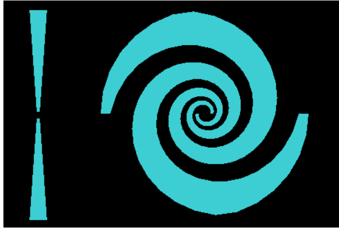
Figure 3.4. Top view of a bowtie antenna (left) and a spiral antenna (right) we try to model (not to scale)
