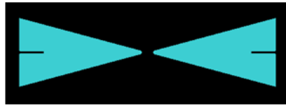
30-degree 110um antenna design with rounded corners
