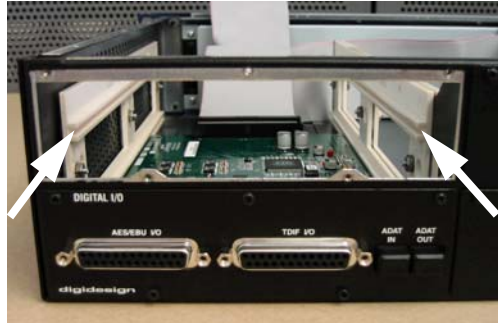
Example of an empty bay. Note guide rails along the inside edge
