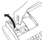
**3** Ensuring the paper is being fed from the bottom of the roll, lower the roll into the space behind the printer.
