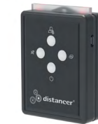
PHYTEC's social distancing tracker enables face-to-face separation measurements within 5-10 cm accuracy
