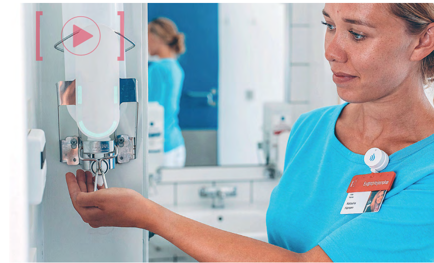
Sani nudge uses staff-worn Bluetooth LE tags and sensors attached to hand sanitizer dispensers to track hand hygiene compliance
