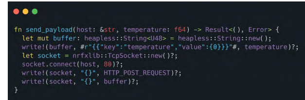
The Rust wrapper around the Nordic socket library uses high level strongly-typed objects, like "TcpSocket" and "ATSocket", which automatically close when they go out of scope and let the developer send formatted data
