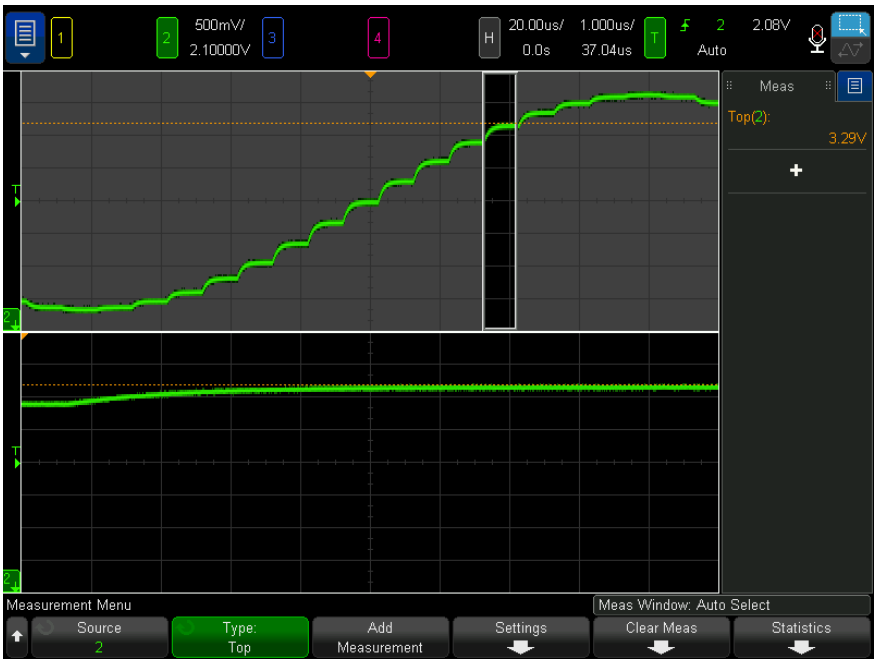
Figure 47 Isolating area for Top measurement
