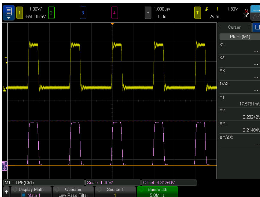
Figure 16 Example of Low Pass Filter
