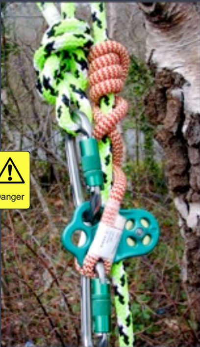
Knotted termination interfering with correct hitch function
