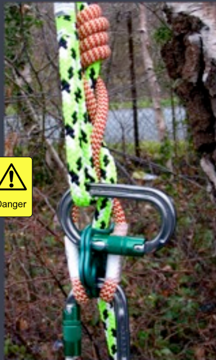
Cross loading of karabiner due to non-captive eye of termination
