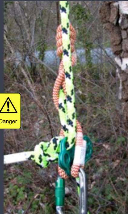
Stopper knot tied behind an attachment hole
