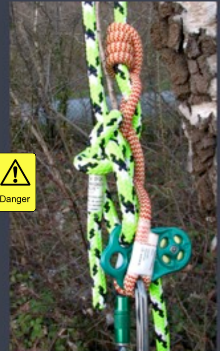
Directly tied into an attachment hole
