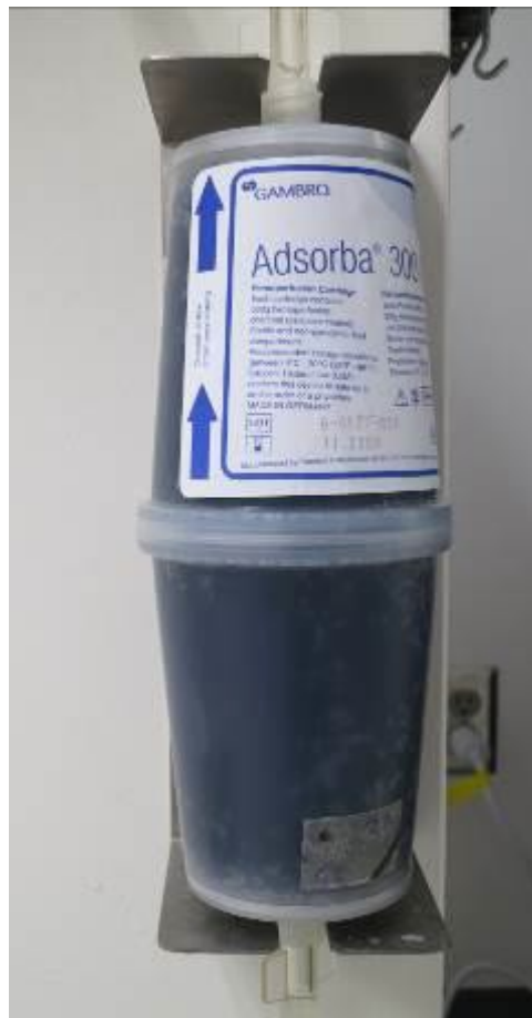
Figure 15b: Confirmation of column installation in bracket
