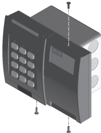
Default: Slide Reader Assembly towards the right to lock.
