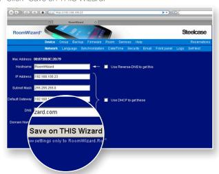
When you change any network settings, you may make the RoomWizard unreachable. If you lose contact with the RoomWizard, reset the IP address manually on the touch screen, and use that IP address to reconnect to the web-based configuration pages.
