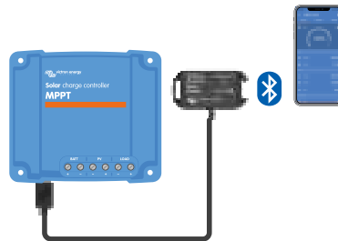
VictronConnect App connection via Bluetooth using a VE.Direct Bluetooth Smart Dongle.
