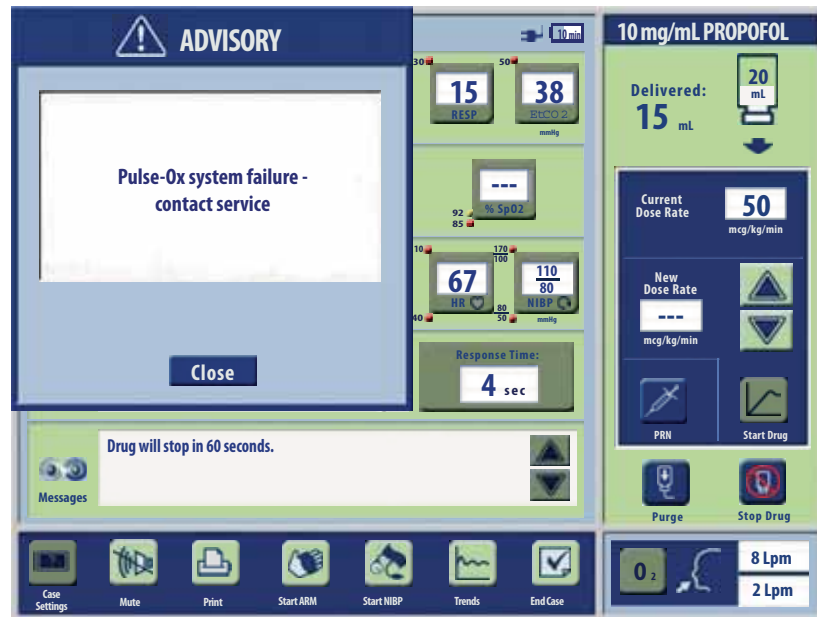
Figure 8-12 PRU Monitoring Screen During Pulse Oximeter Failure Advisory
