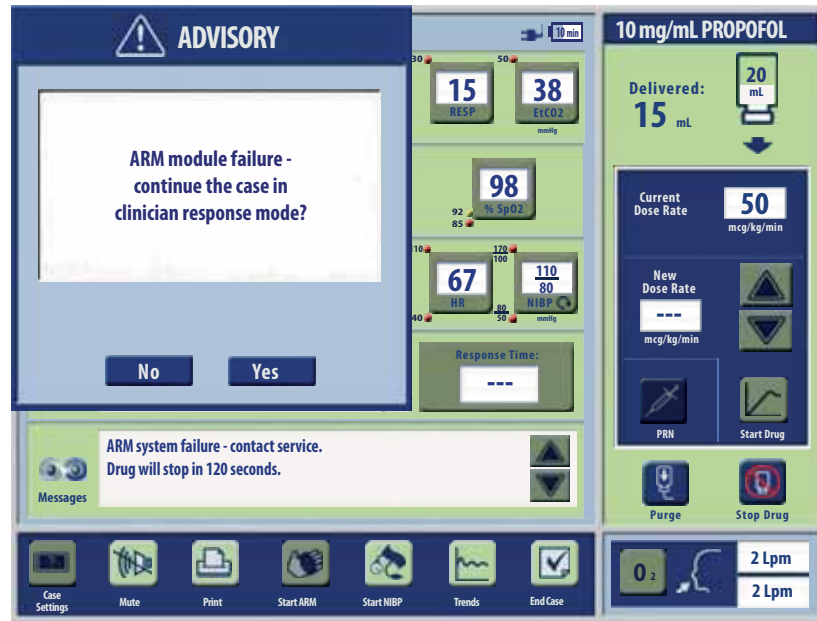
Figure 8-14 PRU Monitoring Screen During ARM Failure Advisory
