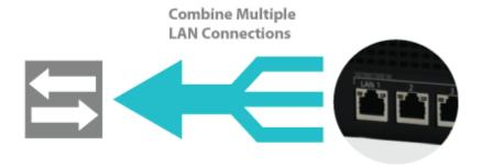
Use 802.3ad to combine multiple LAN connections into a virtual LAN connection. This virtual connection has higher throughput and redundancy in case any single link fails.
