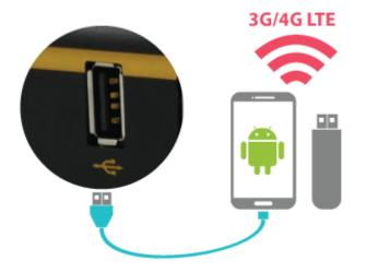
For increased WAN diversity, plug in a USB LTE modem as backup. Peplink routers are compatible with over 200 modem types. You can also tether to smartphones running Android 4.1.X and above.
