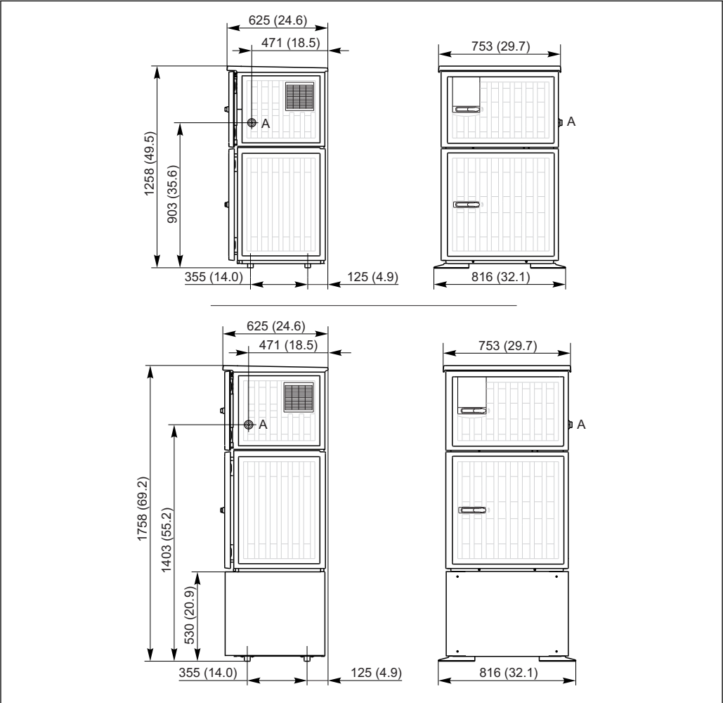
6 Dimensions of Liquistation CSF34 plastic version, without/with stand, dimensions in mm (in) A Suction line connection
