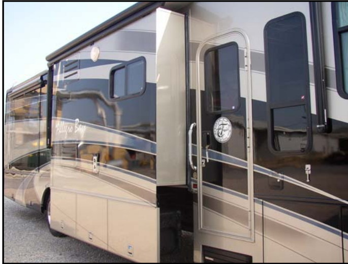
Figure 8-3. Typical Allegro Bay Slide-Out, Fully Extended
