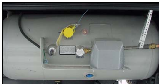
Figure 2-3. Liquid Propane Tank
