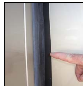
Figure 14-5. Inspecting Slide Out Gasket
