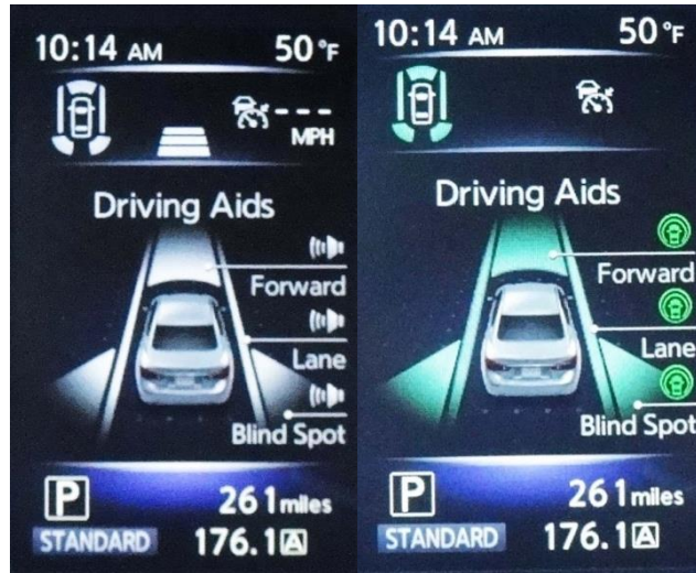
Figure 38. Display for Infiniti Q50 With All Features Off (left) and Lateral Only Active (right)
