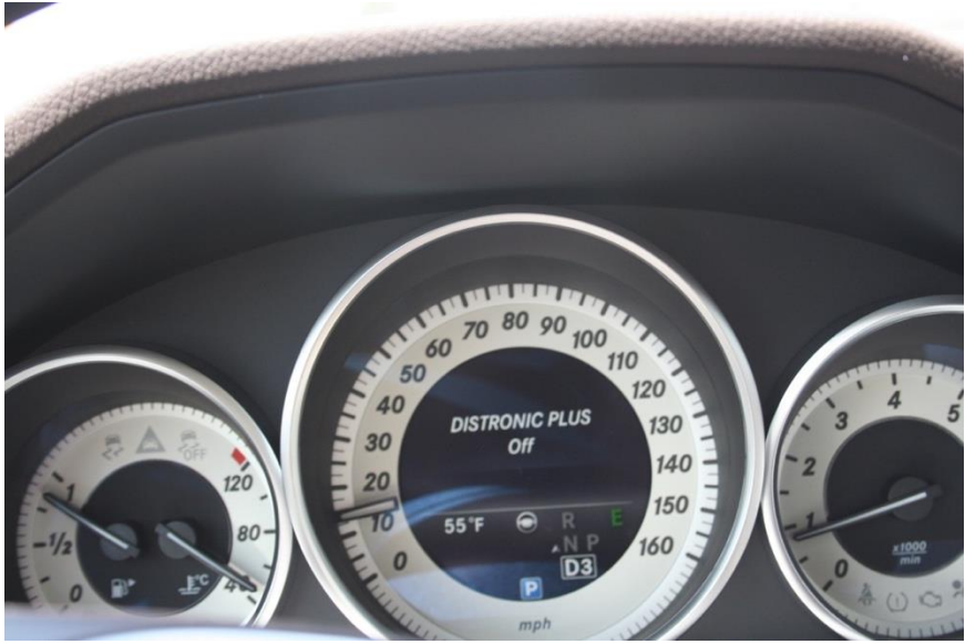
Figure 41. Both Lateral and Longitudinal Systems Deactivated in the Mercedes E350
