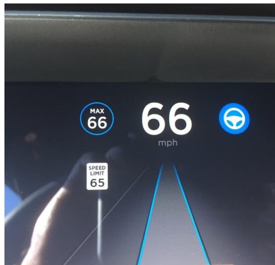
Figure 43. Lateral and Longitudinal Control Systems Both Active in the Tesla Model S
