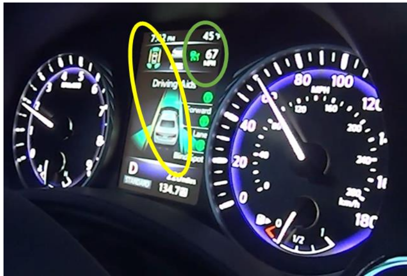
Figure 39. RTI Image (Yellow Circle) With Longitudinal Active (Green Circle) in the Infiniti Q50
