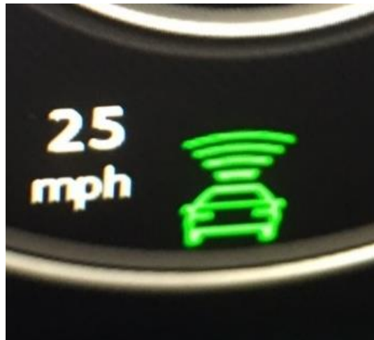
Figure 35. Longitudinal Automation Icon for Audi Q7
