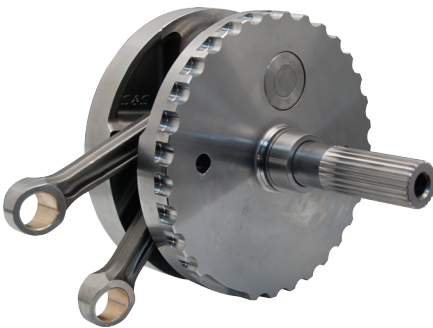
S&S racing flywheels with pressed-in and welded style crankpin. Machined area around crankpin represents the rod clearance option for aluminum connecting rods with large cross section areas.
