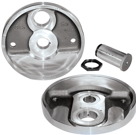
S&S racing flywheels with pressed-in and welded style crankpin. Machined area around crankpin represents the rod clearance option for aluminum connecting rods with large cross section areas.
