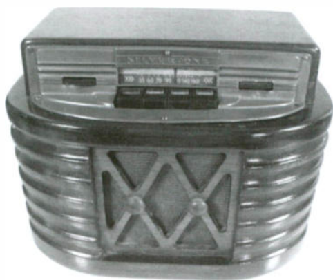
Silvertone model 6320 radio – Manufactured in 1938 by Sears. Cabinet is wood with metal escutcheon. There are four pushbuttons. Chassis is mounted from bottom. Chassis number 101.585. Steven Kirschner, Atlanta, GA
