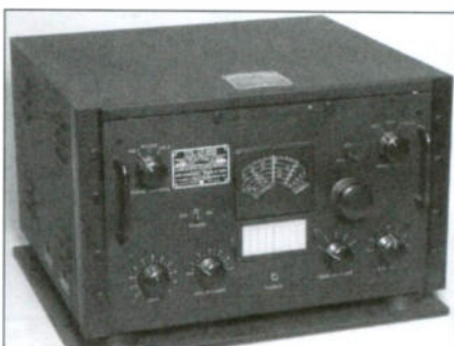
Scott's RCH primary communications receiver.
