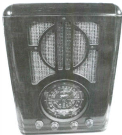
Zenith model 6S229 radio – Attractive 1937 tombstone radio that covered the AM and shortwave bands. There are six tubes in the #5638 chassis. Arnold Bloor, Wheeling, WV
