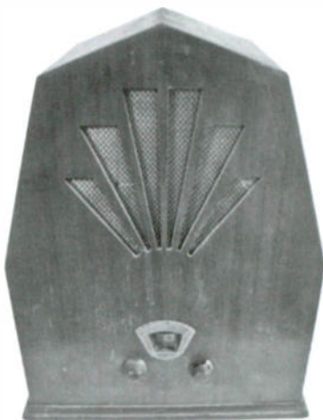
Silvertone model 6320 radio – Manufactured in 1938 by Sears. Cabinet is wood with metal escutcheon. There are four pushbuttons. Chassis is mounted from bottom. Chassis number 101.585. Steven Kirschner, Atlanta, GA
