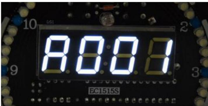
Press the PLUS key again, and the digital tube will display "A002", indicating that the clock is ready to receive the ringtone.
