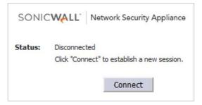
2 Click **Connect**. The WAN interface address and DNS address are assigned by the ISP's DHCP server. SonicOS uses this DHCP IP address for the U0 interface IP address.
