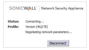
When the connection is active, the **U0/U1 Connection Status** (Connection Manager) displays statistics on the session. Images for a 4G/LTE device and a 3G (PPP) device are shown as follows.
