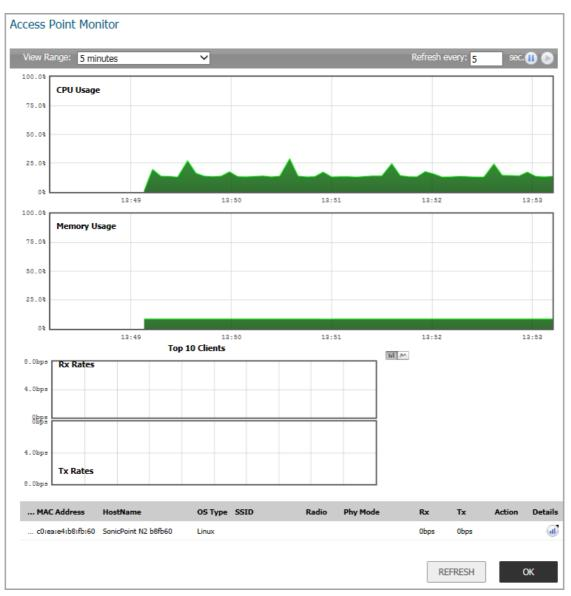
The Access Point Monitor shows system status for the access point. It includes CPU usage, Memory Usage, Rx Rates and Tx Rates.
