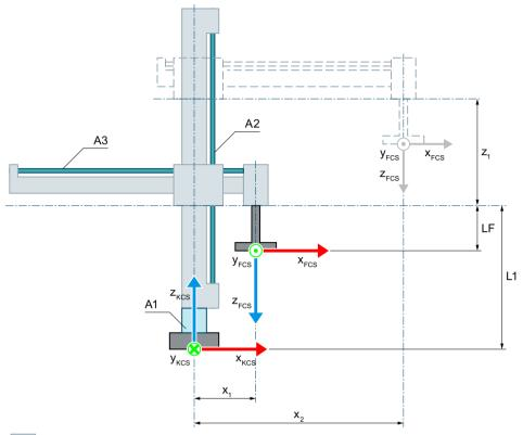
Zero position of the axes A1 and A2
