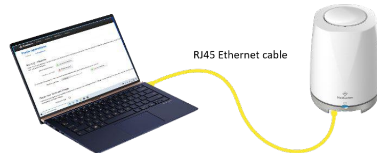
Figure 7 – RJ45 Ethernet cable connecting PC with NS-01
