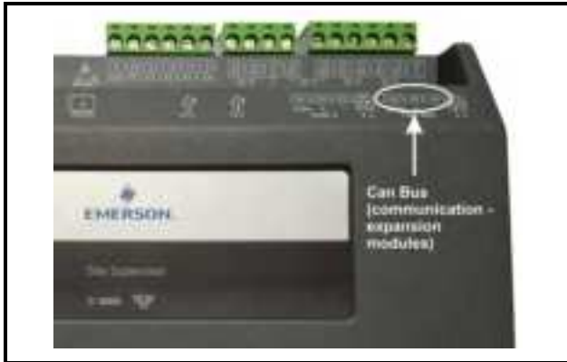
Figure 8-27 - Can Bus Expansion Module
