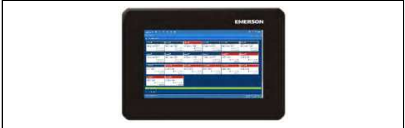
Figure 7-1 - Site Supervisor 10.1-Inch Display
