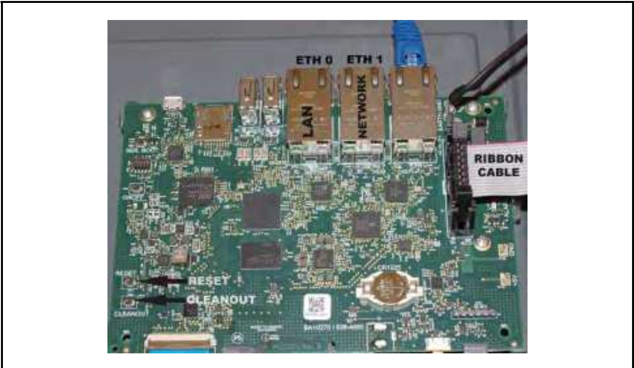
Figure 2-6 - E3 Circuit Board
