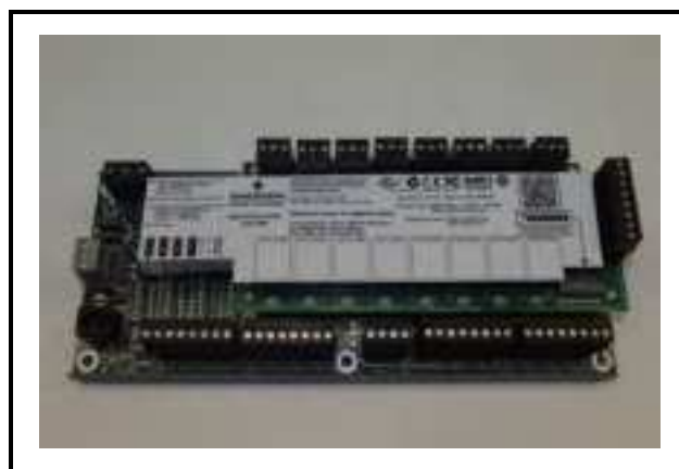
Figure 6-6 - MultiFlex Condensing Unit (CUB)
