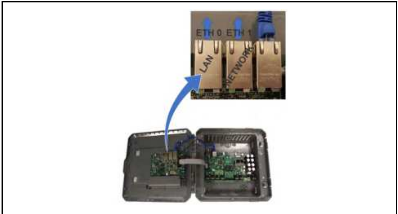
Figure 2-2 - E3 and Ethernet Connection
