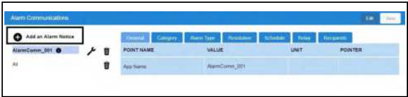
Figure C-17 - Create an Alarm Notice
