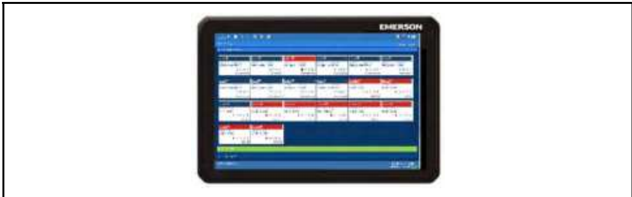
Figure 7-7 - Site Supervisor 15.6-Inch Display
