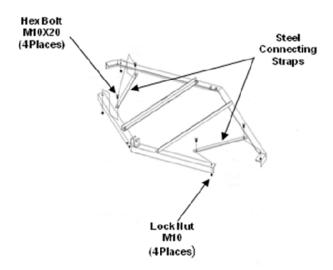
**Step 5** Connect the Tongue to the Main frame using the Hex Bolt and Lock Nuts. Install the Hitch pin and the R pin into Tongue.
