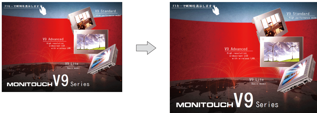
The resolution of 640 × 480 is changed to 800 × 600 when the MONITOUCH model is changed.
