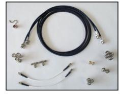
Model 4200-PMU-PROBER KIT: This connection kit consists of standard and custom connectors and accessories used to connect the Models 4225-PMU and 4220-PGU to a variety of common prober stations. It also supports directly connecting the PMU/PGU to the SMU instruments for Flash Memory testing without the need for an external switch. One kit required per PMU/PGU card. Includes:
