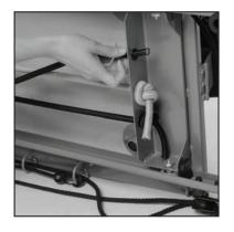
Pull tightly on the cord stretching it to the point that allows you to tie a double knot, and release the cord into place.
