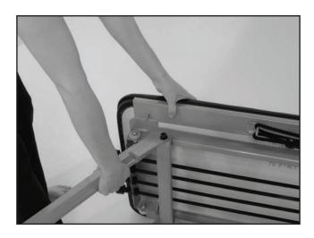
Turn the platform upside down so it is cord side up. Using a crescent wrench and flat head screwdriver, remove the screw that is holding the wheel in place. Replace the old wheel with the new one, add the washer, push the screw through the wheel and tighten with the nut. Do not overtighten the nut and make sure the wheel turns easily.
