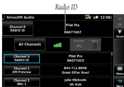
Accessing the SiriusXM Radio ID (Channel 0)
