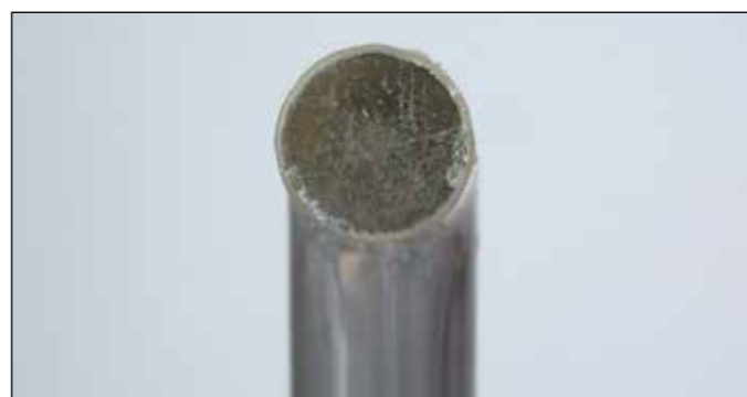
Fig. 6: Damaged 3M™ Elipar™ S10 LED Curing Light used for irradiance testing.
