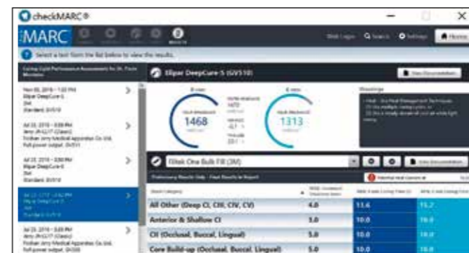
Fig. 3: Results obtained with a new 3M™ Elipar™ DeepCure-S LED Curing Light at 0 mm and at 6 mm distance. The irradiance stated by the manufacturer is also shown. In addition, the overview contains information about potential heat concerns and recommended curing times for selected materials, indications and increment thicknesses.
