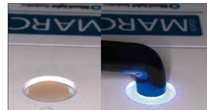
Fig. 8: Determination of the impact of different material shades and translucencies on the light intensity at the bottom: A sample of cured composite of a defined thickness is placed on the measurement spot and the curing light is activated on top of it.
