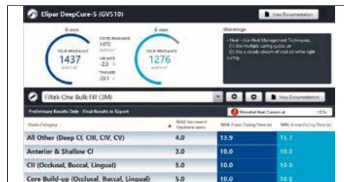
Fig. 5: Test results: There is a slight decrease of the irradiance visible, but it has no impact on the recommended curing times. The impact of the time in service on the performance may be different depending on the product used.
