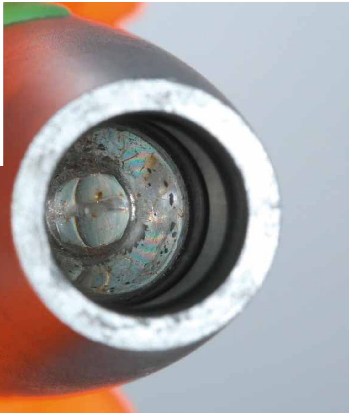
Debris at the interface between the light guide and the body of a light-curing device.
