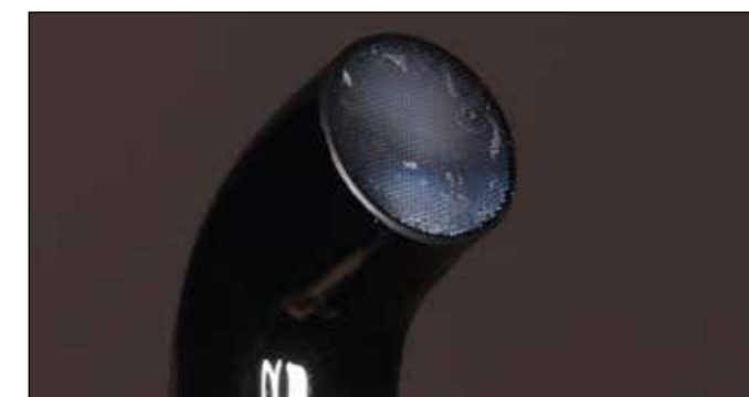
Fig. 4: The same device available for testing after three months of use with some debris on the tip.
