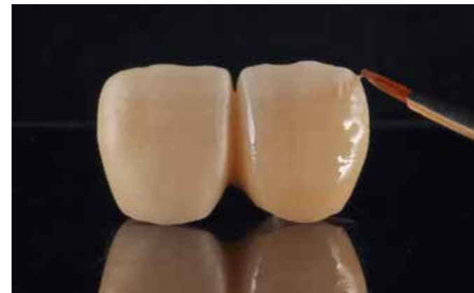
Fig. 4: Splinted crowns made of 3M™ Lava™ Esthetic Fluorescent Full-Contour Zirconia. Milling surface imperfections were removed with dedicated instruments or manual sharp tools made of zirconia or steel to improve the morphology and texture features before sintering.
