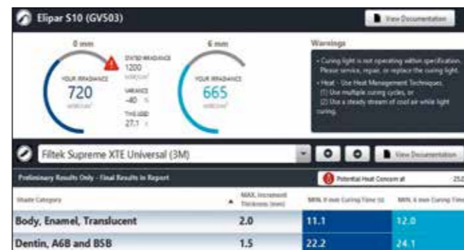
Fig. 7: Test results: Compared to the light intensity indicated by the manufacturer (1,200 MW/cm 2 ), the measured irradiance is 40 percent lower. Such a huge difference usually points towards a problem with the curing light, which is obvious in the present case.
