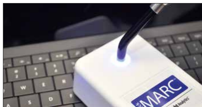
Fig. 2: Spectrometer-based measurement device checkMARC®.
