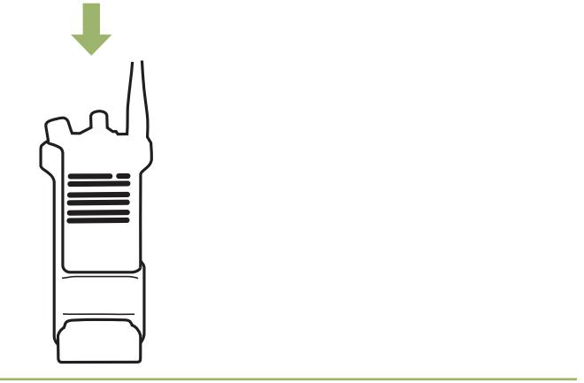
3 To remove the radio from the carry holder, place the tip of your fingers on the ledge of the carry holder.
