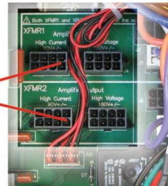
Figure 5.5 – Location of Amplifier High-Voltage Transformer Sockets
