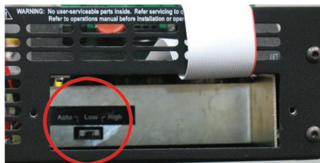
Figure 5.8 – Bi-Level Power Switch Location
