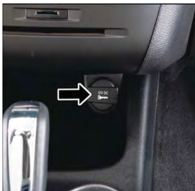
Front Power Outlet
